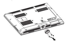
4 Attach the wall-mount bracket with thread ISO M6 type screws only (not included). Make sure that the insertion length (B) of the M6 screws is between 0.39 ~ 0.47 inches (10 ~ 12mm). A shorter length might make the TV wall-mounting insecure. A longer length might create a space between the wall-mount bracket and TV.
